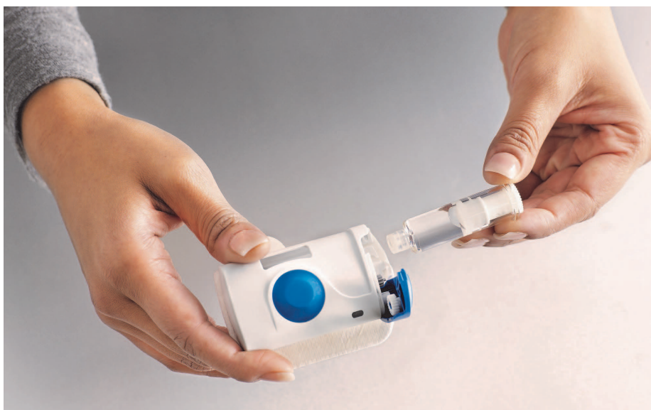
Figure 1: The West SmartDose® electronic wearable injector, designed for patient convenience, incorporates a Daikyo Crystal Zenith® cartridge and can deliver a dose of up to 3.5mL, which may allow for viscous biologics that are sensitive to glass, metal ions and/or silicone oil to be administered over longer periods of time.
