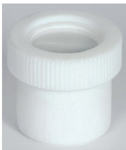
Figure 5: An immersion cell (above) is used with the conventional USP Apparatus 2 fitted with a small volume conversion kit, as shown on the right.
