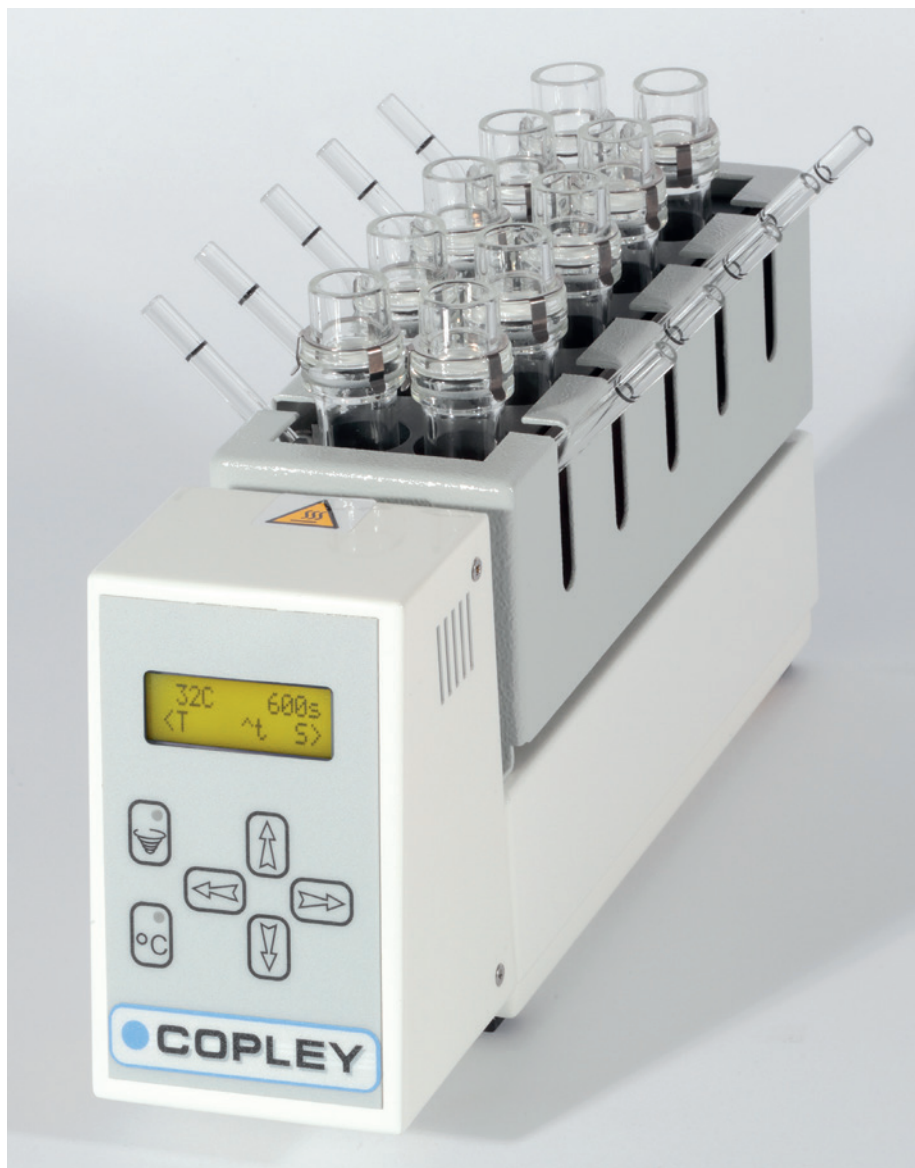
Figure 4: Using a compact heating block for testing is an efficient approach and eliminates the 'spaghetti' of tubing associated with water jacketed designs.
