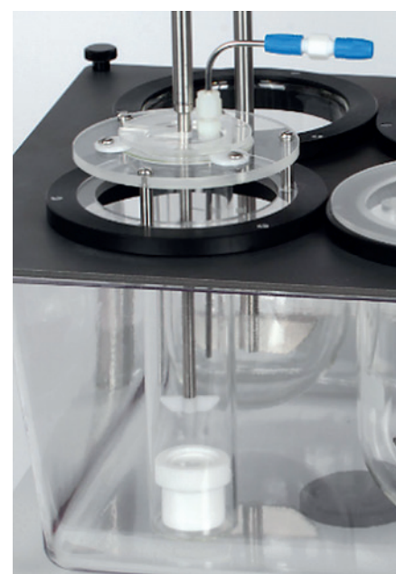
Figure 4: Using a compact heating block for testing is an efficient approach and eliminates the 'spaghetti' of tubing associated with water jacketed designs.
