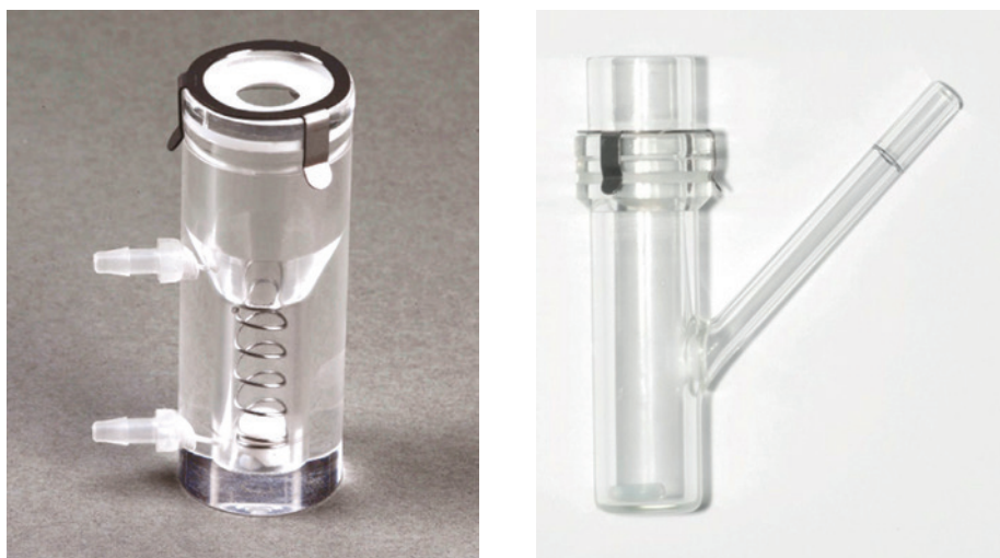
Figure 3: VDC designs such as Model C (right) eliminate the cell leakage/back diffusion issues associated with the double port arrangement of the Model A design (left).
