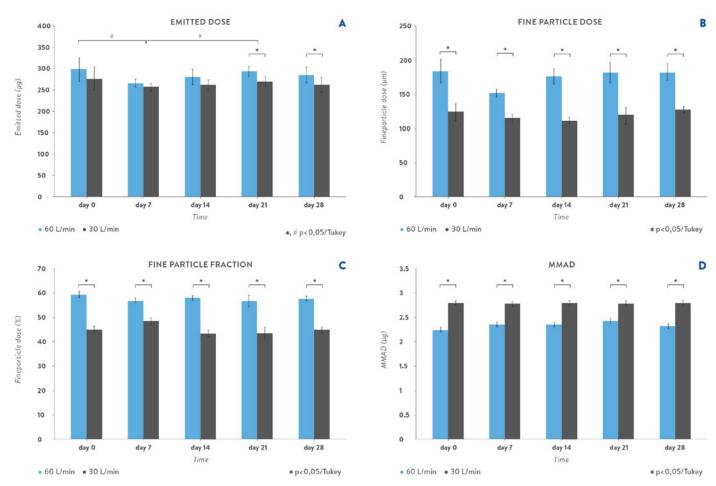
Figure 4: (A) Emitted dose ( $\mu$ g), (B) Fine particle dose ( $\mu$ g), (C) Fine particle fraction (%), (D) MMAD ( $\mu$ m) of salbutamol sulphate at 30 and 60 L/min from a 2-pin standard inhaler (Mean  $\pm$  SD, n=6). \* indicates significance between 30 and 60 L/min. # indicates significance between different time points at 60 L/min.
