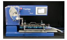
Figure 1: The Vertus can be used with a wide range of collection devices including NGI (shown here), ACI, DUSAs and waste filters. incorporated all elements of inhaler preparation and drug recovery for aerodynamic particle size distribution and dose content uniformity test methods.
