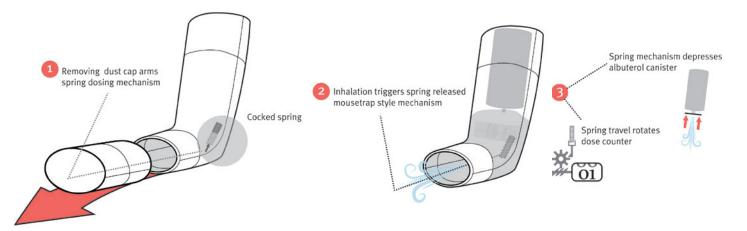
Figure 2: Order of operation for upgrading an automatic-dosing inhaler device.
