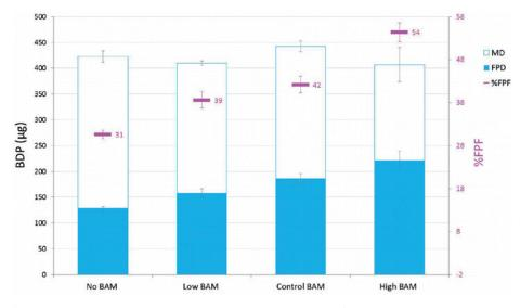
Figure 1: Impaction data shows that dose dispersion performance improves with increasing BAM set pressure; mean values (n=3); error bars  $\pm$ SD.
