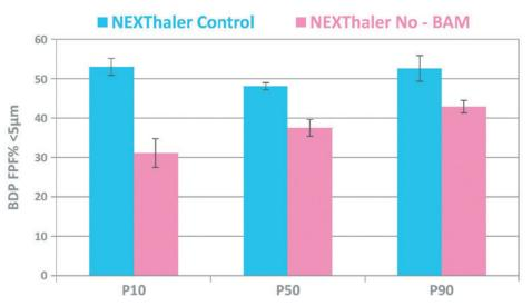
Figure 3: Incorporating a BAM in the DPI device improves the magnitude and consistency of the FPF% across a range of flow rates (n=3).
