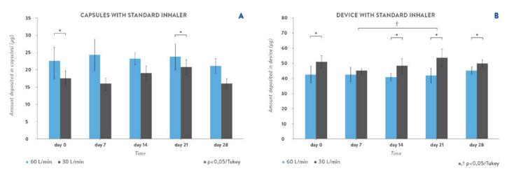
Figure 3: Deposition of salbutamol sulphate remaining in (A) capsules and (B) device, following aerosolisation at 60 L/min and 30 L/min from a 2-pin standard inhaler (Mean ± SD, n=6). \* indicates significance between 30 and 60 L/min. # - indicates significance between different time points at 60 L/min. † indicates significance between different time points at 30 L/min.
