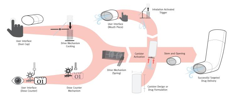
Figure 4: Integration of the inhaler's subsystems.
