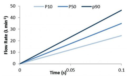
Figure 4: Increase in flow rate between 0 and 0.1 secs for the P10, P50 and P90 inhalation profiles; P90 is associated with the fastest acceleration rate.
