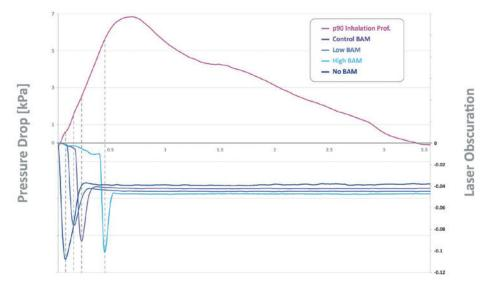
Figure 2: LiveShot dose evacuation kinetics, showing both laser obscuration and differential pressure, provide insight into the enhanced dose dispersion delivered by higher BAM set pressures (n=3).
