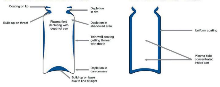
Figure 2: a) Traditional plasma processing does not ensure a uniform coating to internal wall of the canister whereas b) the new plasma process gives a uniform coating to canisters.
