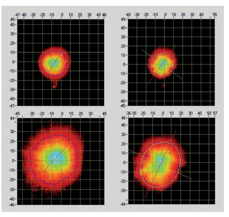
Figure 5: Data from Spray Pattern test at two distances from the actuator orifice.
