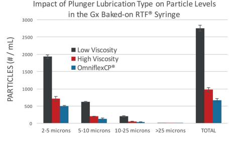
Figure 5: Particle loads by size category as measured by HIAC Royco light obscuration in the Gx Baked-on RTF<sup>®</sup> syringe with various plungers lubrication types. Syringes were aged for 3 months under accelerated conditions and agitated prior to measurement.
