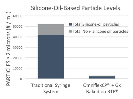
Figure 6: Particle level measurements by MFI in a traditional syringe system (left bar, free silicone on the barrel and a high viscosity siliconised plunger) versus the Gx Baked-on RTF<sup>®</sup> Syringe with OmniflexCP<sup>®</sup> (right). Syringes have been aged under accelerated conditions for three months. The blue portion of the bars represent silicone-oil-based particles and the grey portion of the bars represent other particles.
