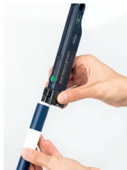
Figure 4: A simple handheld device recognises covert taggants incorporated into plastic materials as anti-counterfeiting and brand-protection measures.
