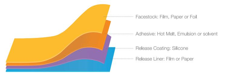
Figure 1: The basic pressure-sensitive label laminate.
