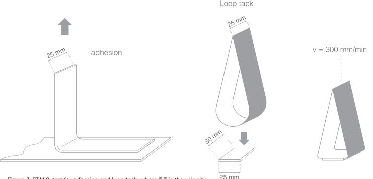
Figure 3: FTM 9, test for adhesion and loop tack, where "V" is the velocity of the tensile tester as it descends onto and then pulls up the test sample.
