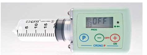
Figure 4: The Crono P is a pump for the infusion of hormones following the body's natural rhythms. The infusion takes the form of a series of boluses at intervals of either 90 or 180 minutes, with a volume which may be programmed from 5  $\mu$ L to 1000  $\mu$ L. The day can be divided into up to three periods, with a different bolus volume programmed for each, such that the circadian and ultradian cycles may be reproduced as required.
