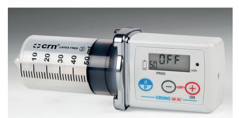
Figure 3: The Crono 50 SC is for the subcutaneous infusion of drugs in the treatment of pain. It has a series of functions for controlling the number and interval between bolus doses, and for verifying how the pump has been used during an infusion. The shot size is  $20 \mu$ L, and the maximum flow rate is 35 mL/h.
