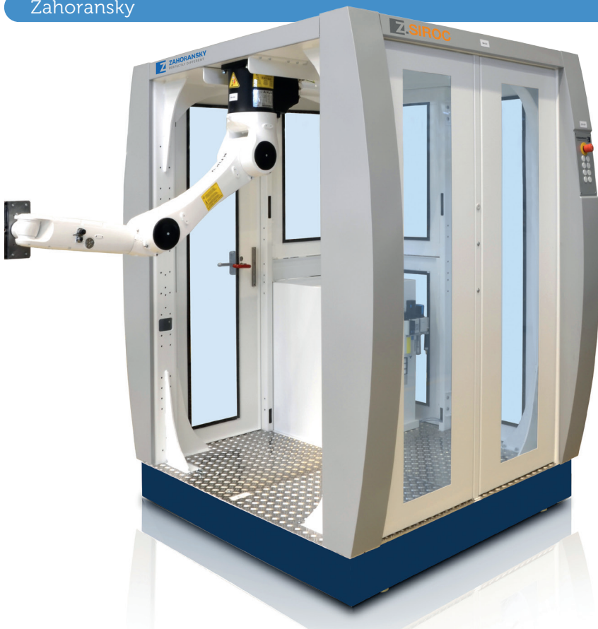
Figure 4: Z.SIROC module mobile extension unit, the heart for the integration of all upstream and downstream processing.
