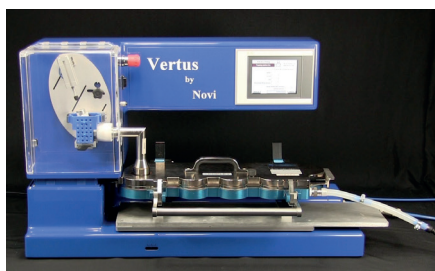
Figure 1: The Vertus can be used with a wide range of collection devices including NGI (shown here), ACI, DUSAs and waste filters.
