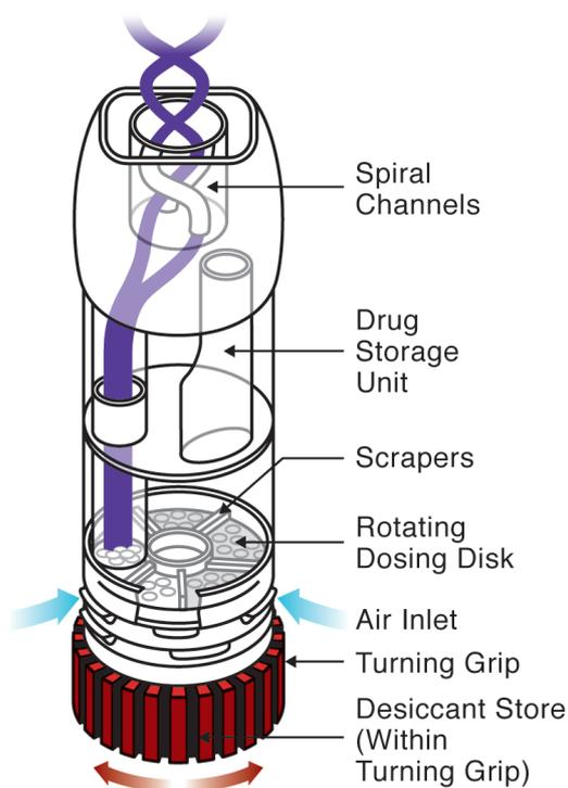
Figure 2: Main components of a typical dry-powder Inhaler.
