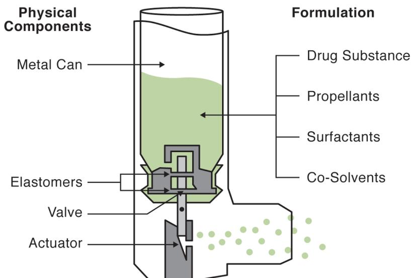
Figure 1: Main components of a typical metered-dose inhaler.
