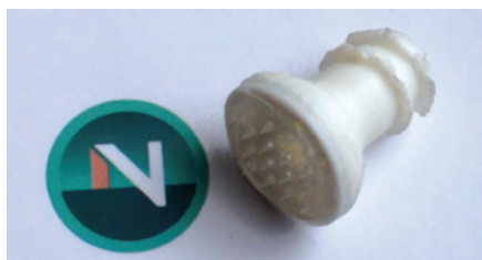
Figure 4: Possible Luer configuration for the microneedle array.
