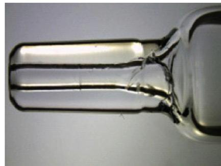
Figure 6: Spiral cracks with low fatigue strength called cone cracks can be found on the area where the cone meets the shoulder.
