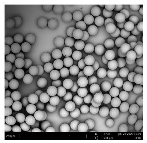
Figure 1: SEM image of 40 µm PLGA particles created with ET4ME.
