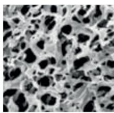
Figure 1: Scanning electron micrograph of nylon membrane filter (pore size 0.22 µm).
