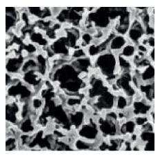
Figure 2: Scanning electron micrograph of a Millipore membrane filter (pore size  $0.22~\mu m$ ) showing a distribution of pore sizes. (Bar in bottom right hand corner of image is  $1~\mu m$  long.)
