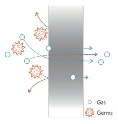
Figure 4: The PureFlow™ technology consists of using the air permeation property of the silicone to allow the air flow and avoid any bacterial penetration.
