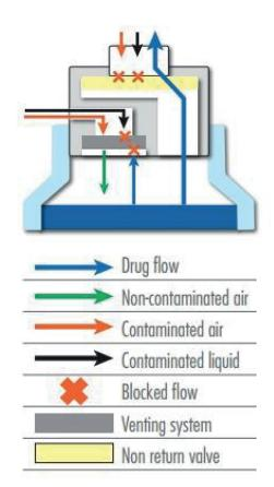
Figure 3: The Novelia® system uses a non-return valve that removes the need to filter the liquid. This makes it possible to use a silicone membrane to filter the air.
