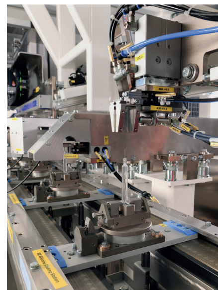
Figure 3: Siliconisation of the needle; special attention is given to ensure that the silicone only comes into contact with the needle only, the syringe body.
