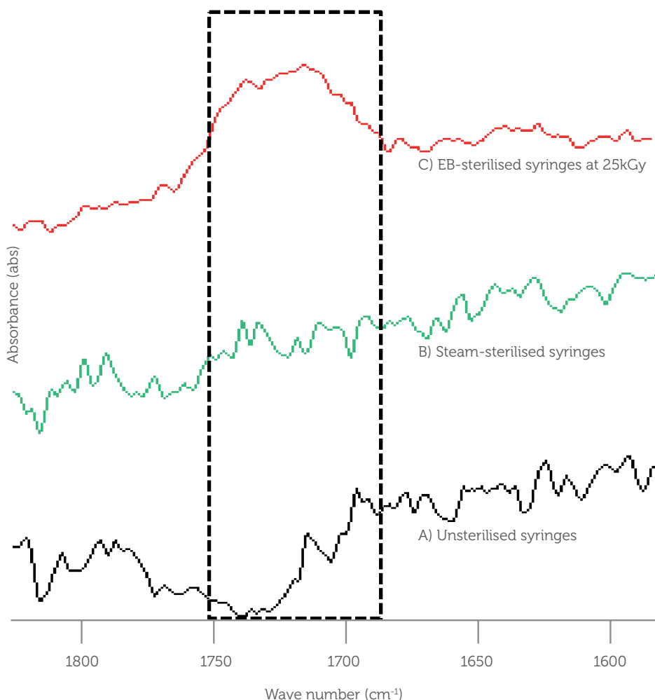
Figure 6: IR spectra of (A) unsterilised syringe; (B) steam-sterilised syringe; and (C) EB-sterilised syringe at 25 kGy. Data are results of a single measurement.
