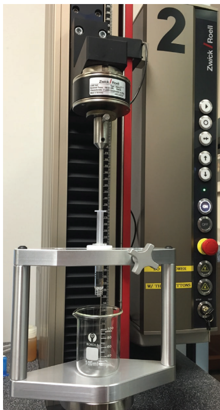
Figure 4: Force-Displacement curves for silicone oil, TriboLink-Si™ and TriboGlide-DS™ lubrication systems acquired using one of TriboFilm’s Zwick Z0.5 Force Testers (left). Break-Loose Force ( F_B ) is defined as the maximum force required to break the static friction of the plunger. Glide Force ( F_G ) is defined as the force required to maintain plunger movement once static friction has been overcome. All samples are 1 mL long glass syringes filled with a 0.05% Polysorbate 80 solution in sterile filtered water. All samples were stored for 12 weeks at 40°C and agitated for 24 hours just prior to characterisation.
