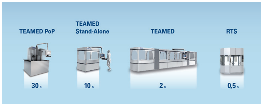
Figure 1: Modular platforms for assembly and function test.
