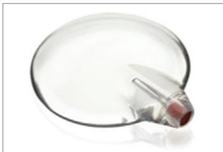
Figure 6: The primary drug container comprises a flexible multi-laminate blister heat-sealed to a rigid base plate, with integrated filling/discharge channel, sealed with a butyl rubber septum.
