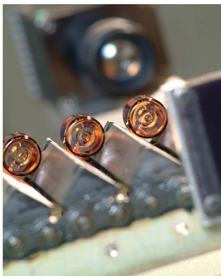
**Figure 1:** Vials are inspected for cosmetic defects.
