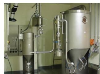
Figure 2: Spray drying apparatus: schematics with main operating parameters (left side) and picture of a GEA NIRO Mobile Minor unit (right side).
