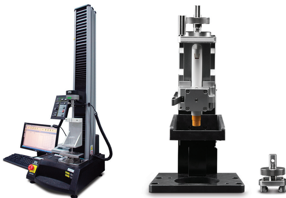
Figure 3: Testing of auto-injectors will require the use of a standalone machine or the use of a standard Instron with customised fixtures and a vision system.
