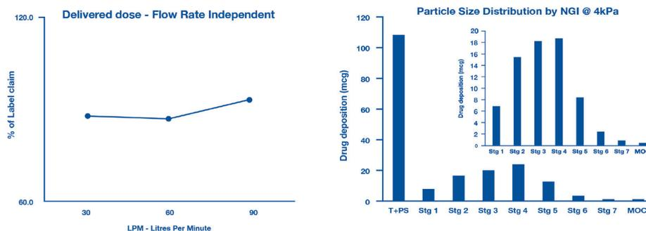
Figure 5: *In vitro* performance data of PowdAir Plus device for a marketed salbutamol capsule-based formulation.
