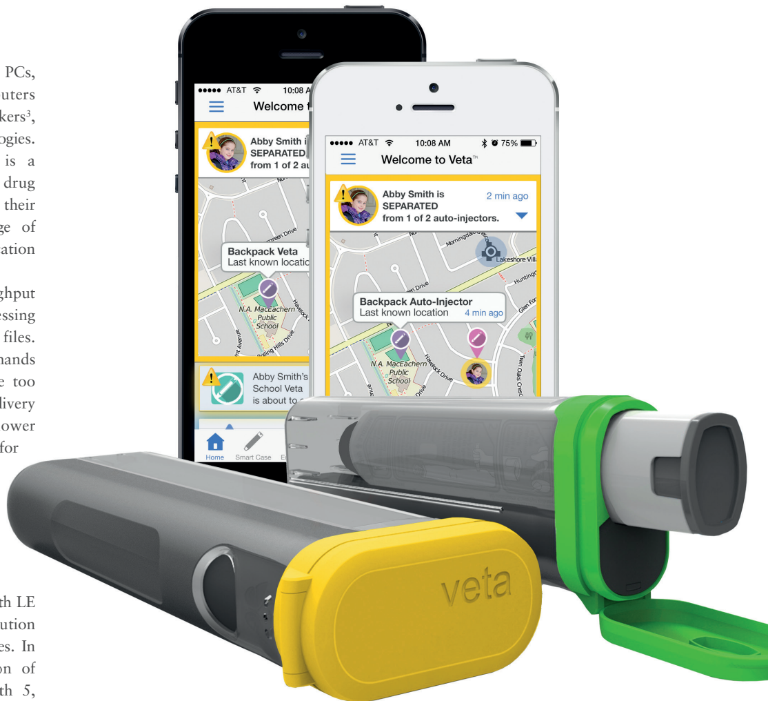
Figure 3: Aterica's Veta EpiPen smart case employs low-power wireless connectivity to notify the user in the event they become separated from the device.
