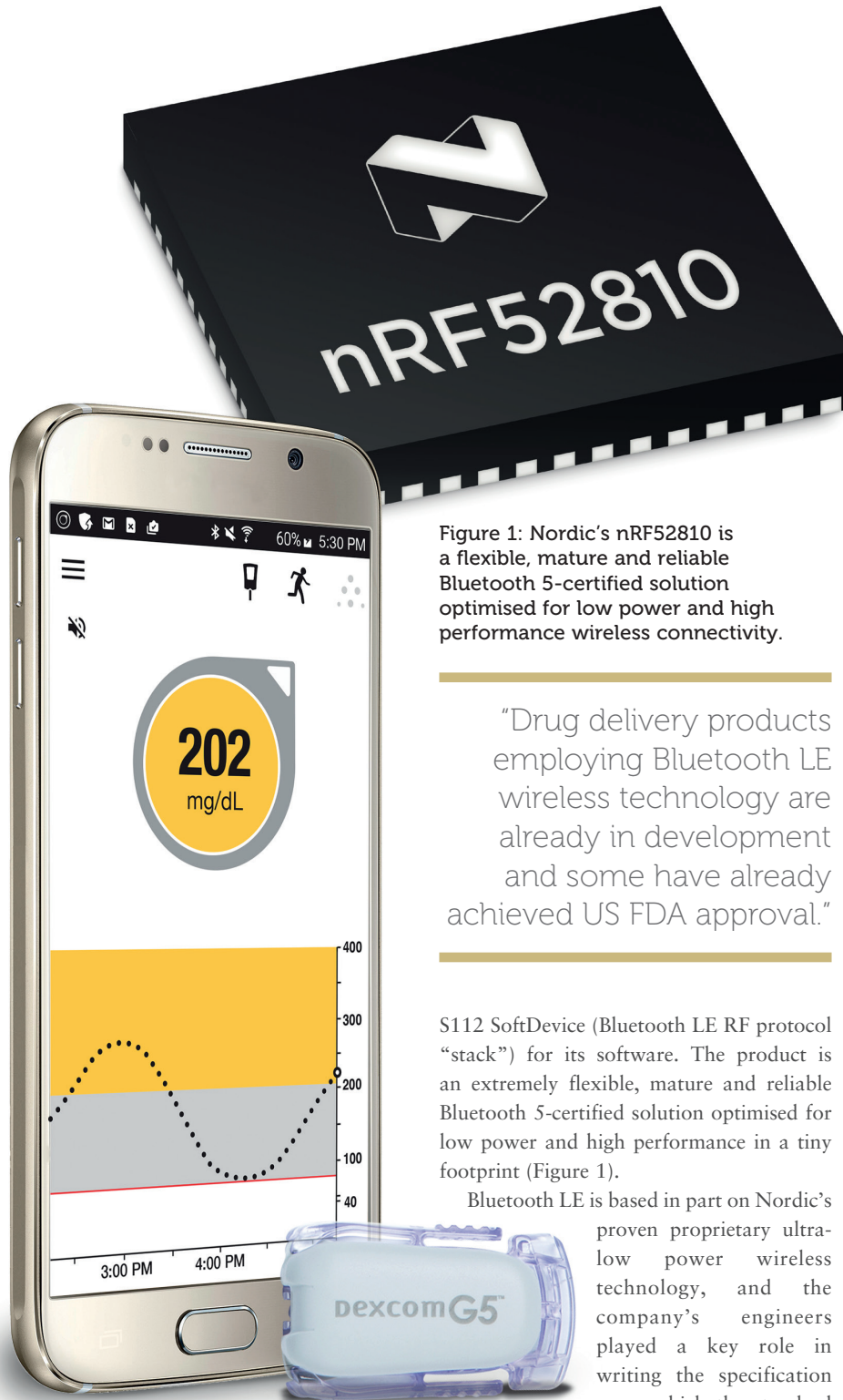
Figure 2: The FDA-approved Dexcom G5 Mobile CGM transmits blood glucose readings to a smartphone using Bluetooth Low Energy wireless technology.
