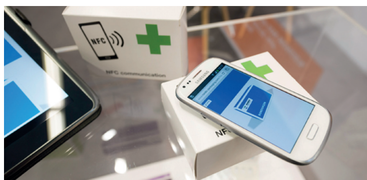
Figure 2: Rondo uses NFC chips integrated in the pack to improve patient communication. The NFC chip transmits its information as soon as a ‘read’ terminal is within range.
