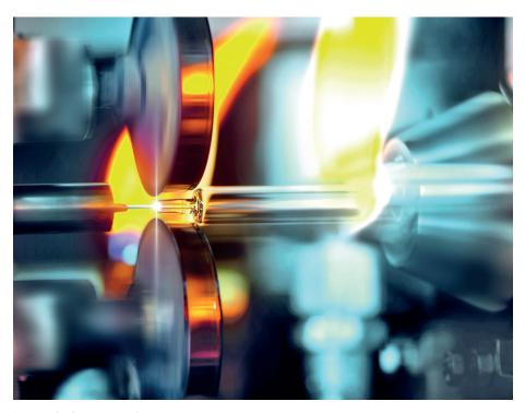
Figure 2: Cone bore forming step.
