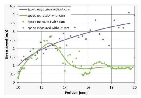
Figure 6: Measured needle insertion with and without a cam.
