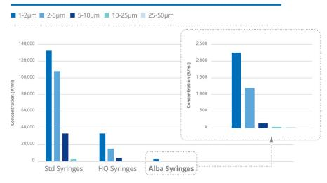
Figure 1: Alba syringe particle release performance in comparison with standard and high quality syringes.
