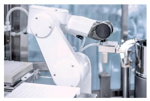
Figure 4: Fully automated robotic filling of syringes. (© Bosch/AbbVie)
