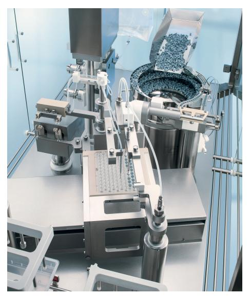
Figure 2: Complete combination filling line for nested containers. (© Bosch)
