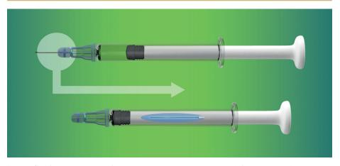
Figure 2: After the user performs an injection, they hear and feel a click when the dose is fully delivered, and then the needle is retracted back into the plunger rod and the barrel of the syringe.
