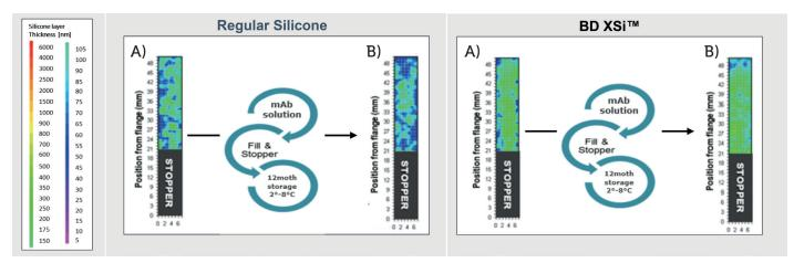
Figure 2: BD Neopak™ XSi™ maintains coating integrity and gliding performance compared with regular silicone, both at baseline (A) and at 12 months (B), measured by reflectometry.
