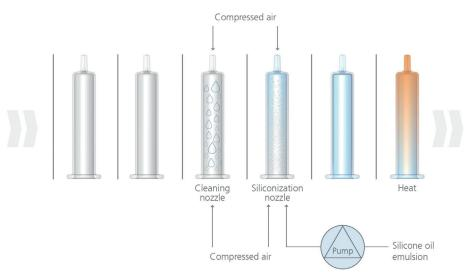
Figure 3: Baked-on siliconisation processing steps.
