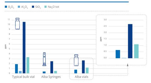
Figure 2: Alba vials inorganic extractables release performance in comparison with bulk vials and Alba syringes.
