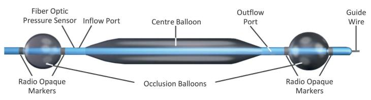
Figure 1: Schematic of the Occlusion Perfusion Catheter™.
