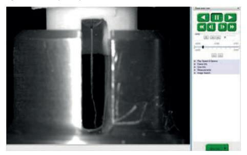
Figure 8: Start of injection just after needle insertion with a cam.
