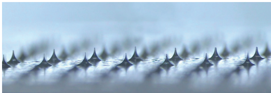
Figure 2: Microscope image showing the protrusions of a dissolving microstructure array.
