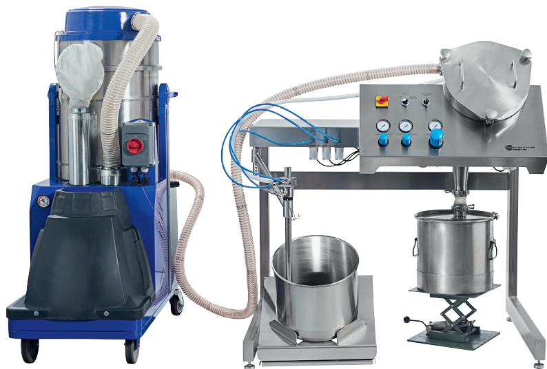
Figure 1: The spiral jet mill micronises particles by accelerating them in high gas flow causing them to collide and fragment.
