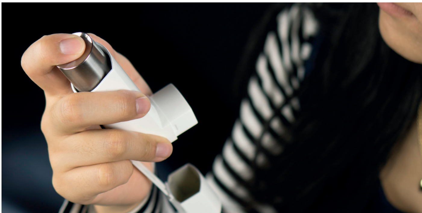
Figure 1: MDI training device designed to replicate an actual MDI's form factor and operation while providing the user with multisensory feedback.
