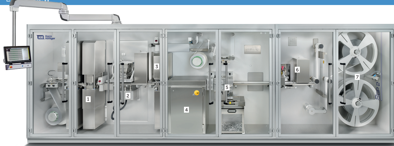
Figure 3: Machine for the manufacture of powder-filled blister strips: 1) Forming station; 2) Membrane filler; 3) Sealing station; 4) IPC X-ray module; 5) Longitudinal cutting; 6) Printing with camera control; 7) Winding.
