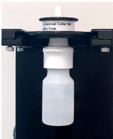
Figure 3: In vitro volume delivery test with Advancia nasal pump.
