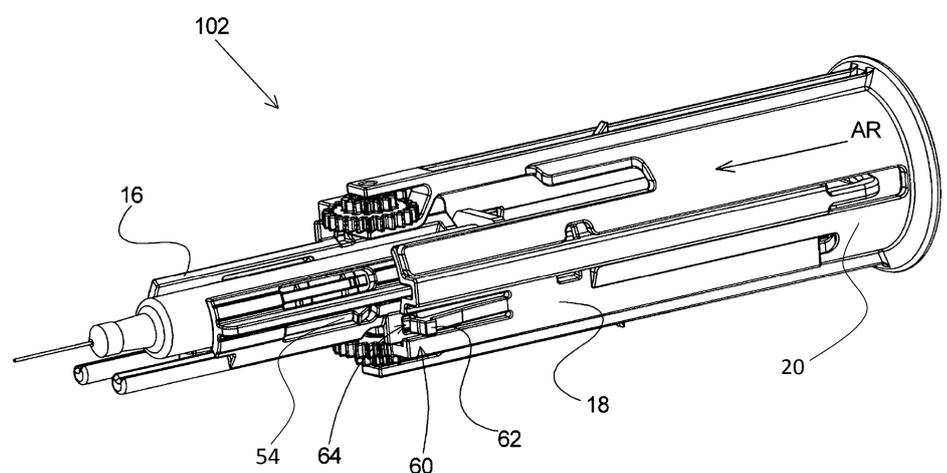
Figure 2: Patented injection device with toothed gearing during application.
