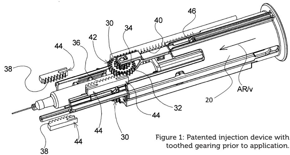
Figure 1: Patented injection device with toothed gearing prior to application.
