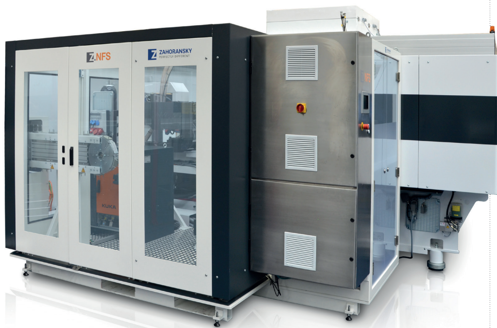
Figure 1: The Z.BLIZZARD manufactures ready-to-fill prefillable syringes from COCs/COPs with very high autonomy.
