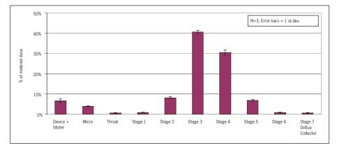
Figure 3: NGI performance of a DPI formulation containing 400µg apomorphine hydrochloride in a 2mg formulation, delivered from the Aspirair active DPI device.
