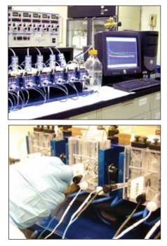
Figure 5: Top: Ussing absorption unit; Bottom: Slider with the intestinal tissues being mounted between the side-by-side compartmental unit of the Ussing system.
