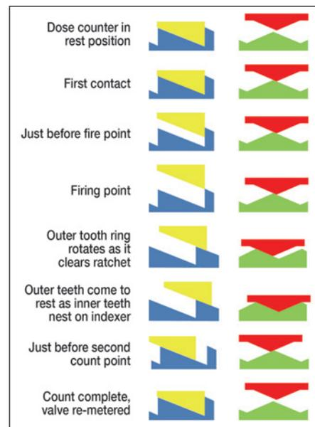
**Figure 3: Diagrammatic representation of the split-count principle.**
