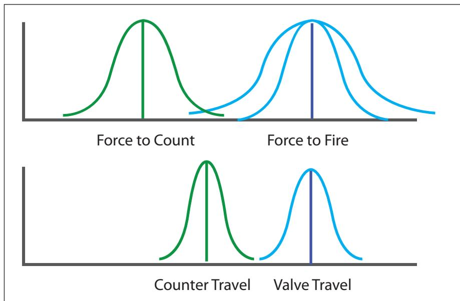
**Figure 1: Schematic representing variability of count-fire points using force to fire versus valve displacement mechanisms.**
