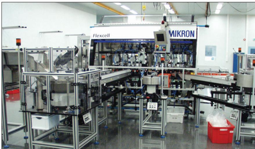
**Figure 6: DPI automated assembly equipment.**
