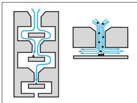
**Figure 1: Multistage cascade impactors size fractionate a sample, particles with sufficient inertia breaking free of the airstream and impacting on the collection surface at specific stages.**
