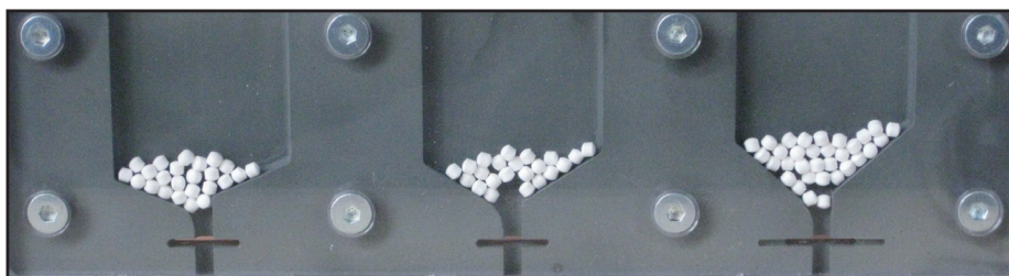
Figure 6: The phenomenon of arching which blocks the device's exit channel.
