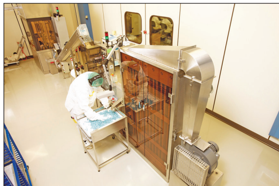
Figure 4: One of two Tillotts Services Bosch GKF 1500 and Shionogi S100 production lines.
