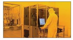
Figure 6: Nanoject<sup>™</sup> manufacture and assembly takes place in ISO class 5 down to ISO class 3 clean rooms.
