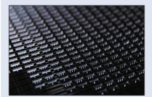
Partial view of an eight-inch wafer, with chips of one and three microneedles.
