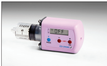
Figure 4: The Crono FE is a pump for the treatment of infertility. For this treatment the drug must be delivered as a series of boluses, and the Crono FE may be programmed to administer boluses from 5-1000 \mu l at intervals ranging from 5-300 minutes.
