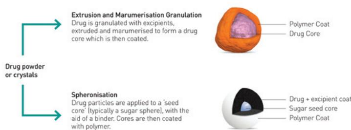
Pellet technology used for controlled release formulations.
