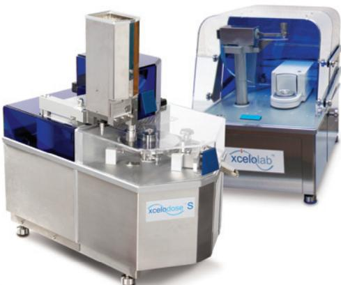
Xcelodose® 600 S precision powder micro-dosing system and Xcelolab™ powder dispenser
