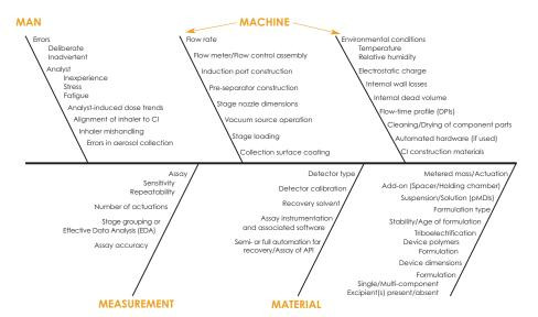
Figure 3: The complexity and manual nature of cascade impaction means that that are many potential sources of variability.<sup>5</sup>
