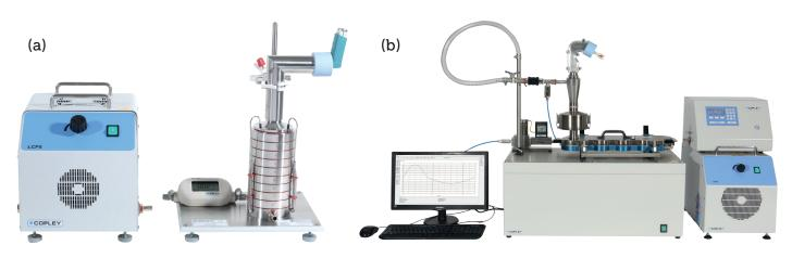
Figure 2: Test set-ups for APSD measurement depend on the purpose of testing such as: a simple ACI set-up for QC for MDIs (a), or an NGI set up for enhanced IVIVCs for DPIs (b).
