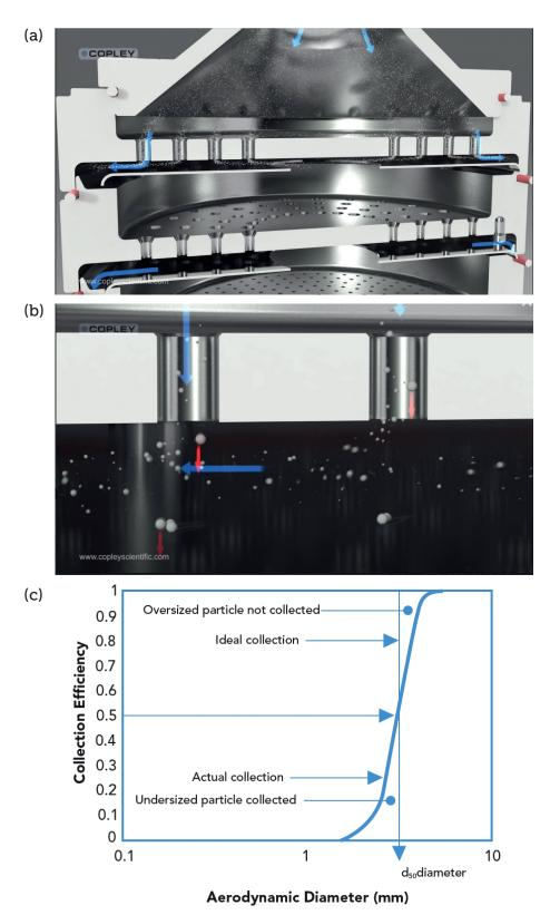
Figure 1: As sample is drawn through the stages of a cascade impactor (a), progressively smaller particles acquire sufficient inertia to break free of the prevailing air flow and impact on the associated collection surface (b). At any given flow rate each stage therefore has a defined cut-off diameter, the D50 of the collection efficiency curve (c).
