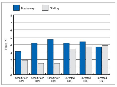
Figure 2: Break-Away and Gliding Forces after Storage.
