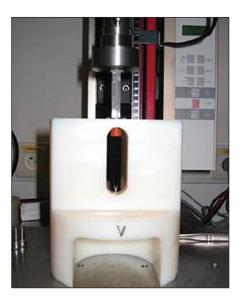
Figure 3: PBSI, Build-Up for Compression Testing.
