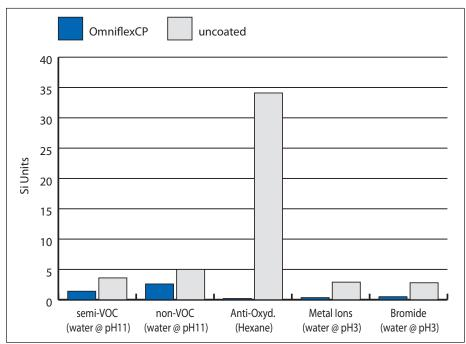
Figure 4: Extreme Conditions Extractables and Leachables Testing.
