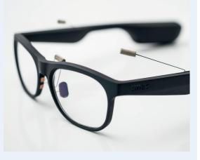
concept which integrates wireless eye-tracking technology into a standard pair of eyeglasses. The smart glasses use electro-oculograms, which measure the electric potential across particular points on the skin around the eyes during eye movement. The glasses use five dry-contact electrodes developed by Datwyler.
