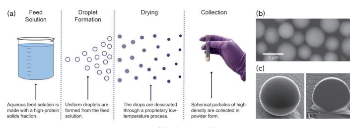
Figure 1: Elektroject™ microparticle production process (a), microparticles (b), and a cross section of a single microparticle demonstrating non-porous morphology (c).
