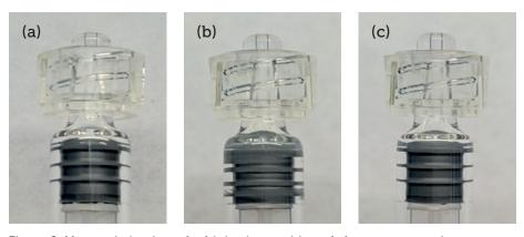
Figure 2: User variation in end-of-injection position of plunger stopper: just bottomed out (a), forced into the shoulder region (b), and retracted having been forced into the shoulder region (c).
