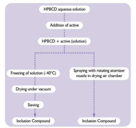
Figure 3: Preparation of inclusion complex in aqueous solution.
