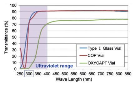
Figure 4: Graph comparing UV transmission properties of OXYCAPT™ with COP and glass.
