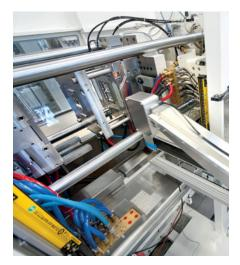
Figure 3: A detailed view: The Z.NFS needle separating system can separate 4– 32 needles or cannulas with up to 12 cycles per minute. Currently, diameters from 0.2 mm and lengths up to 45 mm can be processed.
