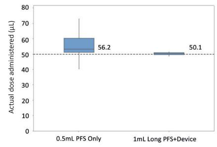
Figure 3: Boxplot with 95% CI of ophthalmologists (n=21) attempting to inject 50  $\mu$ L with a 0.5mL PFS only and device + 1 mL "long" PFS (n=100) in a lab setting.
