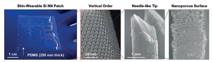
Figure 2: Photograph of a representative Si NN-patch (left) and magnified images of the tips and the nanoporous surface.
