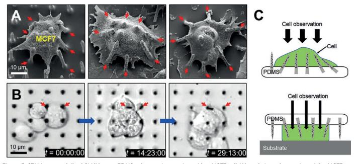
Figure 3: SEM images of tilted Si NNs on a PDMS substrate interacting with a MCF7 cell (A), real-time observation of the MCF7 cells through the transparent PDMS substrate (B) and schematic illustrations of the possible injection schemes from either top or bottom of cells (C).
