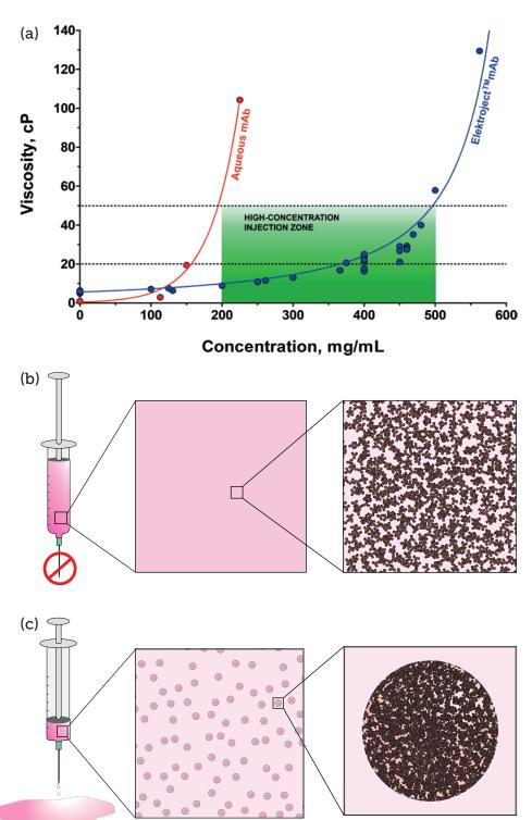
Figure 2: Elektroject<sup>™</sup> enables high concentrations of biologics at low viscosity. Graph's x-axis shows protein concentration for aqueous mAb and particle concentration for Elektroject<sup>™</sup> mAb (a). Intermolecular forces drive viscosity and protein degradation at high viscosity (b). Elektroject<sup>™</sup> formulations physically reorganise protein solutions into reversible suspensions to reduce viscosity (c).
