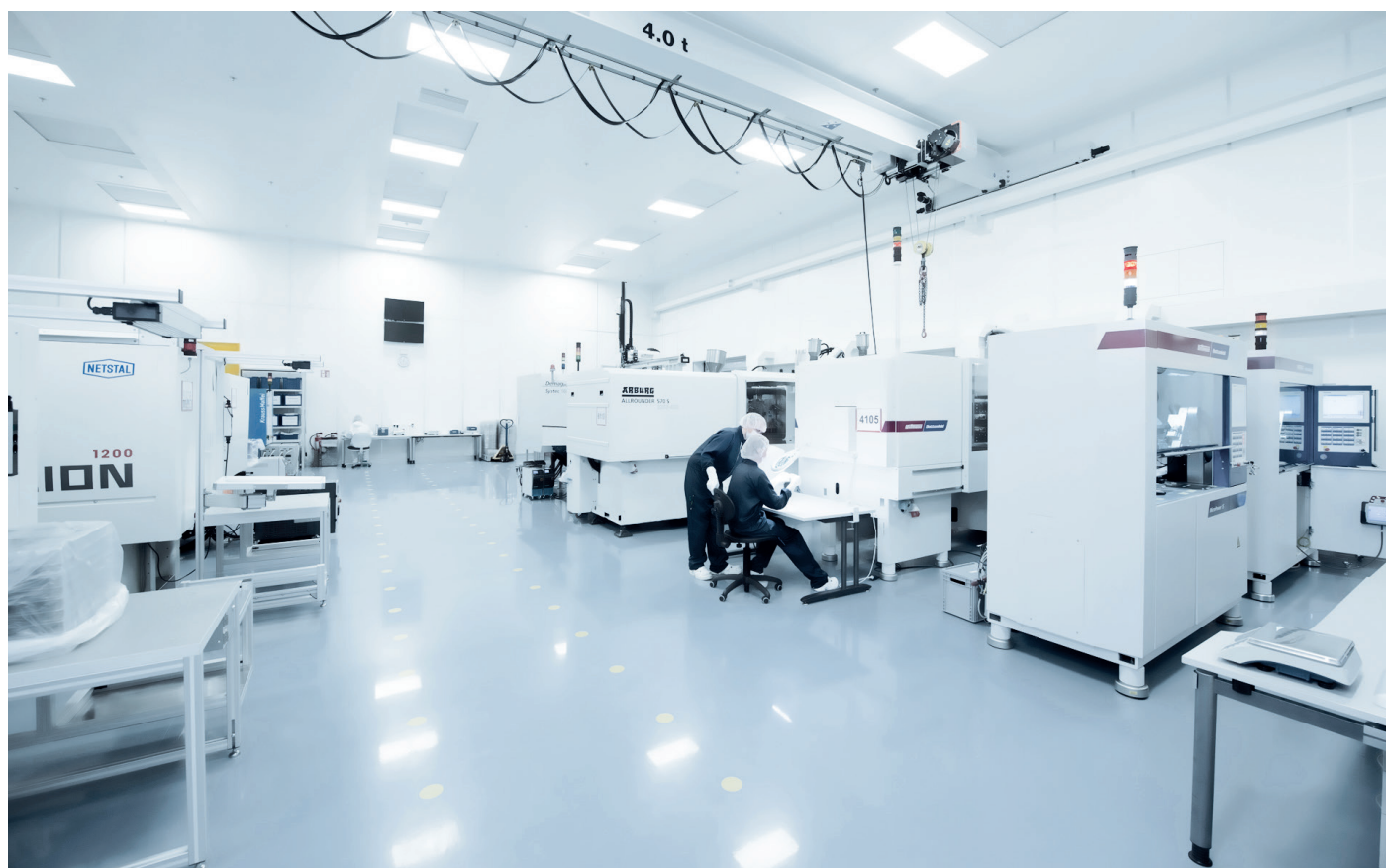
Figure 2: Gerresheimer's small batch production facility has a class 8 clean room in accordance with DIN EN ISO 14644-1.
