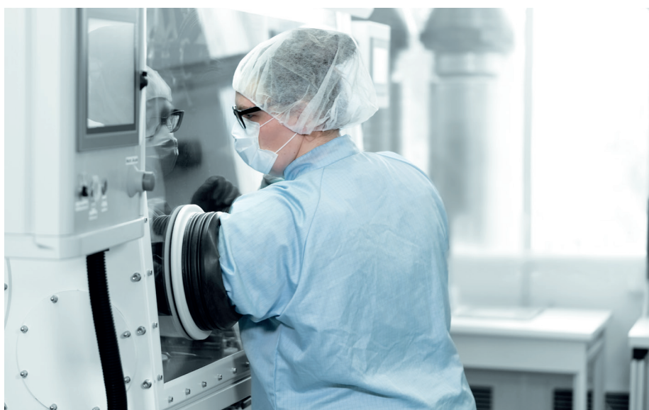
Figure 1: The small batch production facility has a room with a vacuum for filling toxic materials and, depending on the requirement, it may be done in a protective atmosphere.
