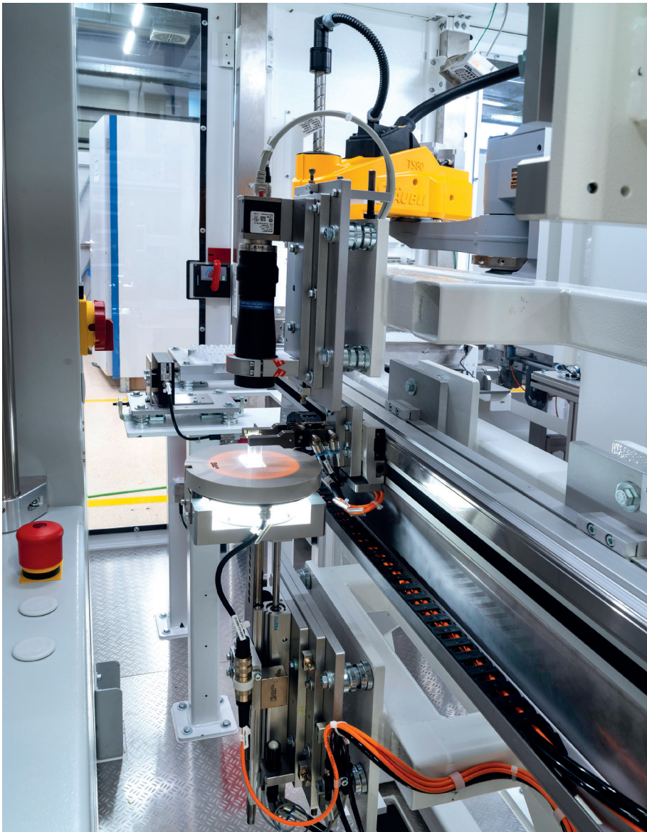
Figure 2: More than ten camera systems can ensure continuous monitoring, as well as an integrated 100% X-ray system for quality assurance after assembly.
