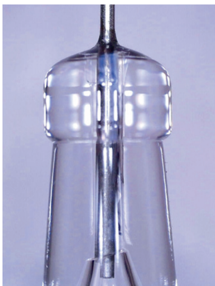
Figure 1: UV-cured adhesive bonding needle to syringe.
