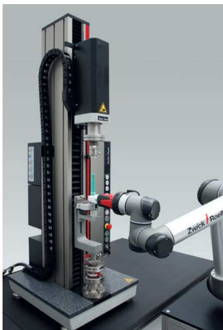
Figure 1: Fully automated breakaway force and glide force.
