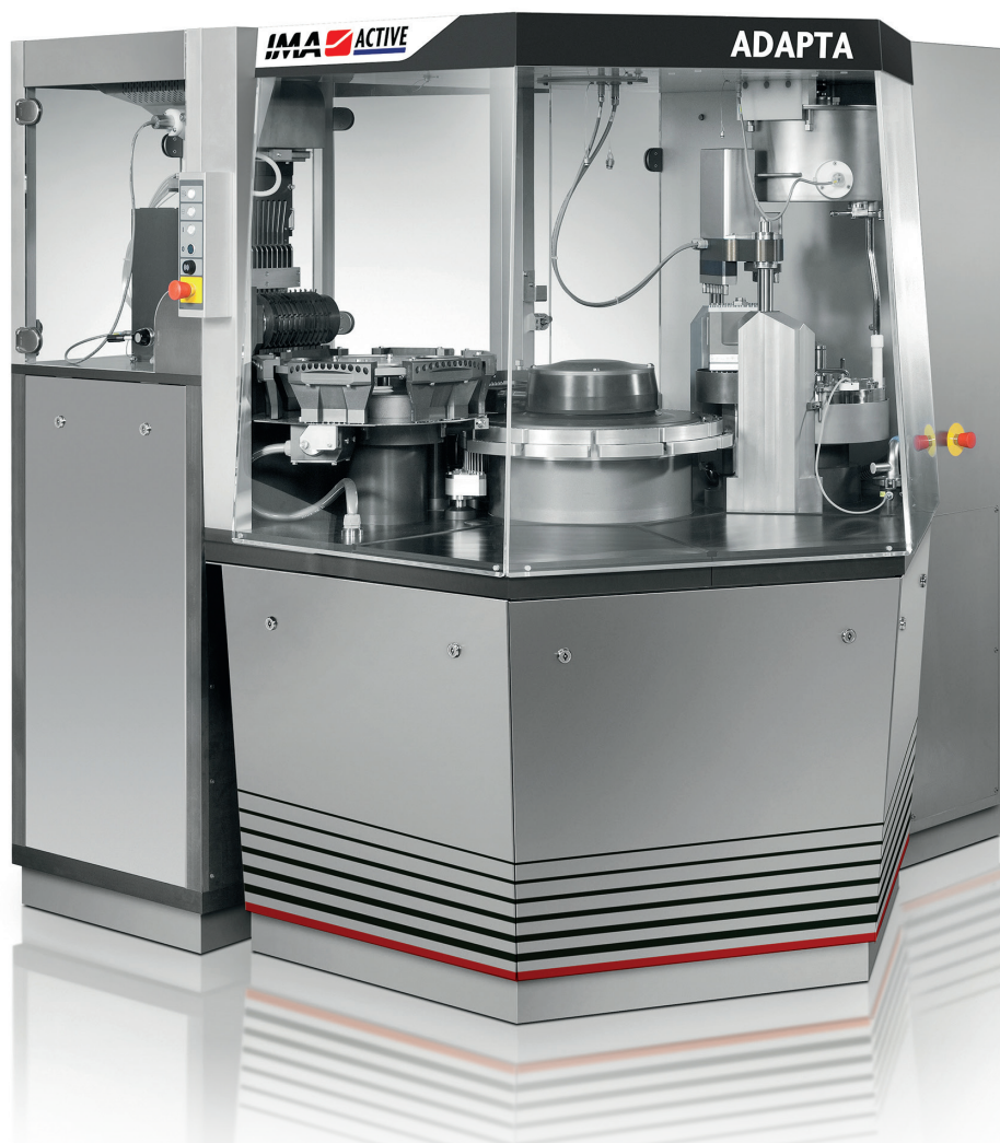
Figure 1: Adapta® 100, IMA's dosator capsule filling machine with 100% gravimetric net weight control.
