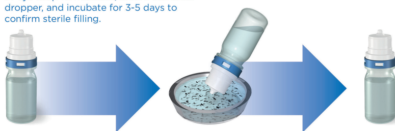
Figure 2: New microbiological challenge test (TSIT 2.0) as performed by Aptar Pharma, showing the principle of the TSIT 2.0 (A), and a test to check potential contamination of next dose (B).
