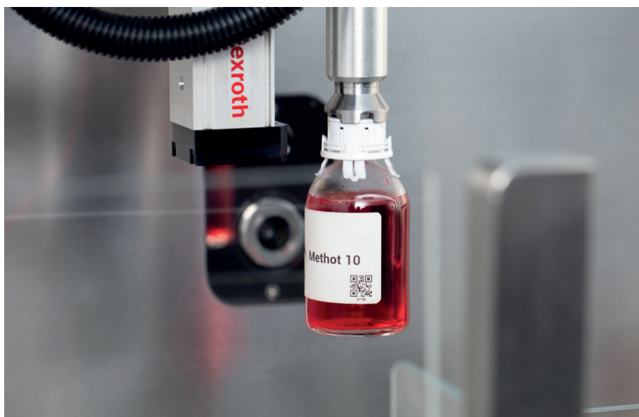
Figure 4: The Equashield PRO vial-grabbing mechanism and verification system.
