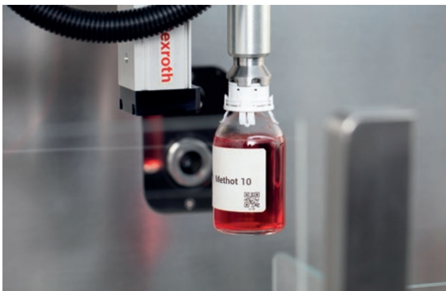
Figure 4: The Equashield PRO vial-grabbing mechanism and verification system.
