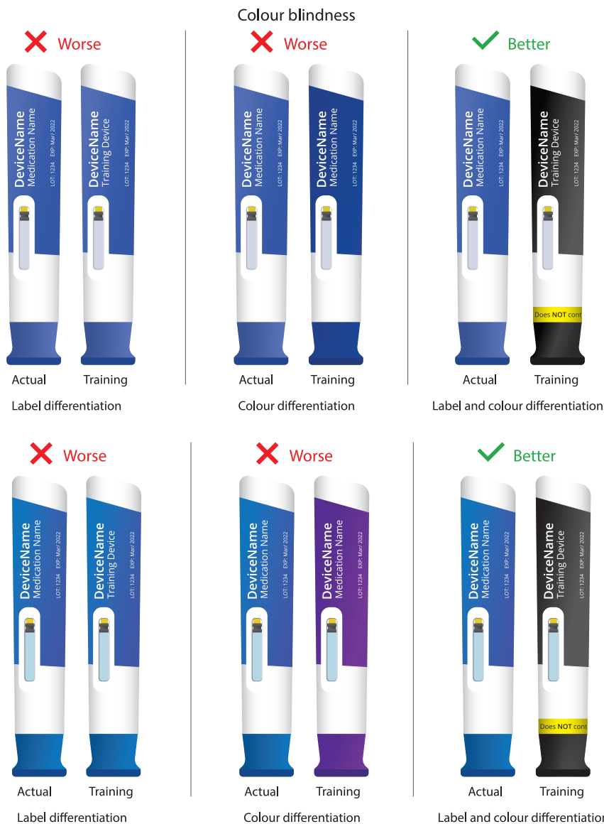
Figure 2: Colour and labelling variations impact users' ability to differentiate between training and actual devices, including visual deficiencies such as red-green colour blindness.
