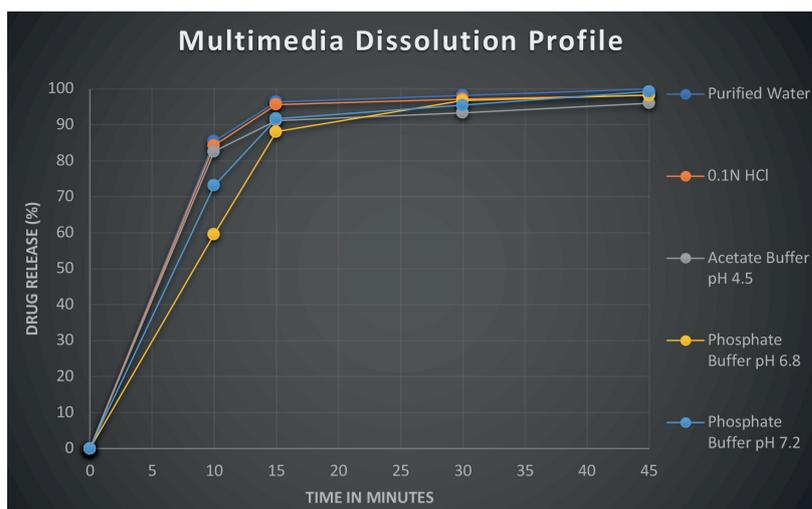
Figure 1: Dissolution profile of acetaminophen in ACGcaps™ H+. (Apparatus used: USP Type 2; Volume: 900 mL; Speed: 50 rpm; Time interval: 10, 15, 30 and 45 minutes.)
